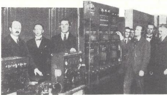
EIGHT VOICES PLAY LEAPFROG ON TWO WIRES.—Four men in Melbourne held independent conversations with four others in Sydney on one pair of wires yesterday. Between the two cities there will now be five telephonic channels instead of two. On the extreme left is the Postal Director (Mr. Brown) supervising a test of the apparatus before the demonstration. With him are Messrs. S. H. Witt, H. S. Robertson, G. H. Schmidt, R. G. Bussell and J. S. Jammer, departmental engineers.
