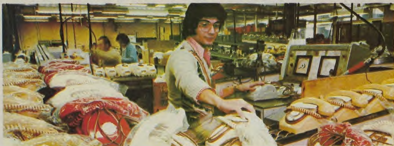
New telephones get a final testing on the production line.
