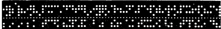
THIS IS THE 'COMMON LANGUAGE' WHICH LETS MAN CONVERSE WITH COMPUTERS. PAPER-TAPE. Contains information in machine readable form.
