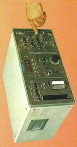
"ANDO" Test Set being Used for Trio's testing on Regenerators
