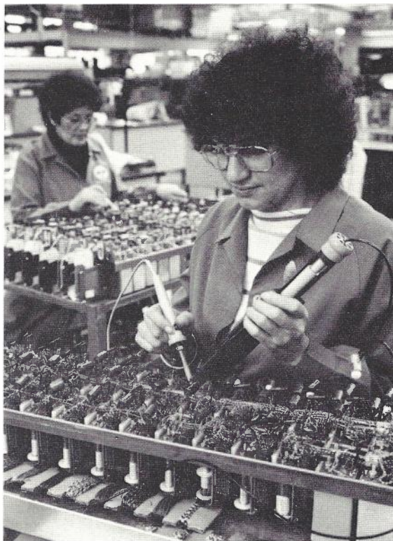
Modification of Relay Sets for REMO at Melbourne Workshops
