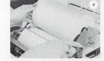
4 Stretch the paper and make the edges of the paper run parallel to the edges of the roll. Swing the lever of the paper holder towards the back of the machine. Tear the paper off along the paper cutter. Operate the UNLOCK switch to return the teleprinter to operation. Press the LOCAL switch. When the LOCAL indicator lamp glows, carry out a test from the keyboard to ensure the paper feeds correctly.
