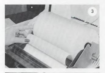
$3\,$  Insert the paper over the spring-loaded bar behind the platen then under the paper cutter.
