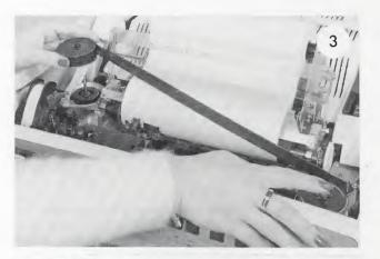
3 Hold the spools with the new ribbon in position (See sketch on the underside of the lid for details on path).
