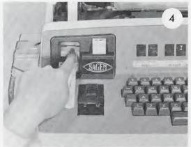
3 Free the tape holder of the punch by pressing the associated lever.
