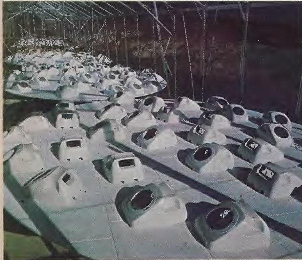
ABOVE LEFT: Telephone casings in a sunlight test for colour fastness, plastic stability. CENTRE: A chilling test for telephone cables. ABOVE RIGHT: A simulated lightning test to ensure safety of rubber boots, mats used by lines staff.
