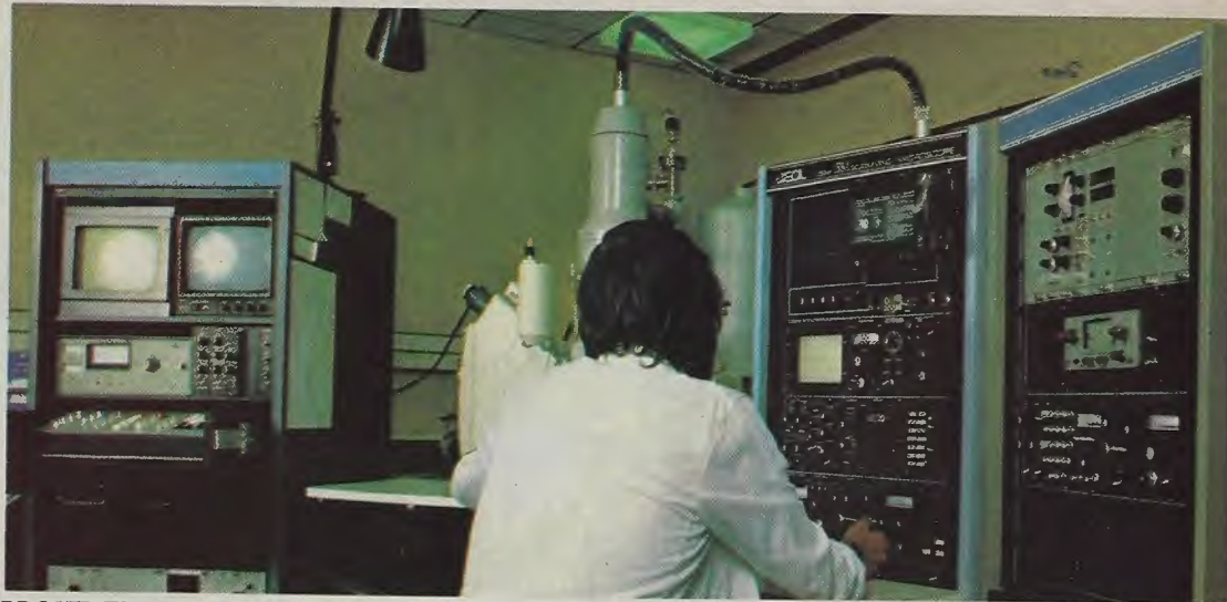
ABOVE: Electron microscope used to view fibres. RIGHT: A cross-section magnified 1200 times. BELOW: Fibre cable (right) carries 10 times the traffic of the copper.
