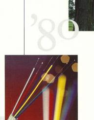
1981 Experimental optical fibre link installed between two exchanges near TRL for testing and evaluation. TRL recommended use of single mode optical fibre for the long distance network, making Telstra one of the first telcos in the world to install single mode optical fibre networks in the mid to late 1980s.
