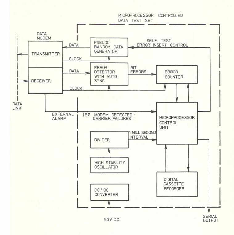
FIG.1 BLOCK DIAGRAM OF DATA TEST ARRANGEMENT
