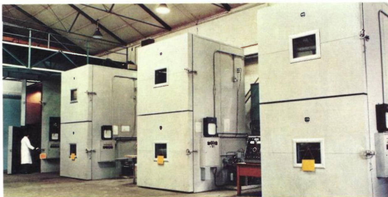
ENVIRONMENTAL CHAMBERS — THE FOUR CHAMBERS CAN PROVIDE TEMPERATURE RANGES OF -40^{\circ}\text{C} to 93^{\circ}\text{C} AND RELATIVE HUMIDITIES FROM 11% TO 100%
