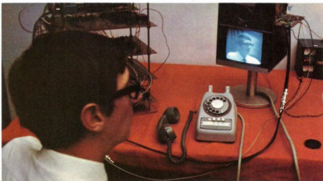
T.V. PHONE SHOWING A SELF-VIEW OF THE SPEAKER, THE CONTROL TELEPHONE AND AT LEFT, THE EXPERIMENTAL DPCM ENCODER
