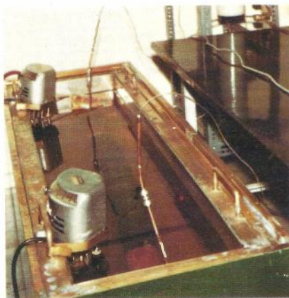
ELECTROLYTIC CELL FOR MEASUREMENT OF MOISTURE CONTENT OF NITROGEN
