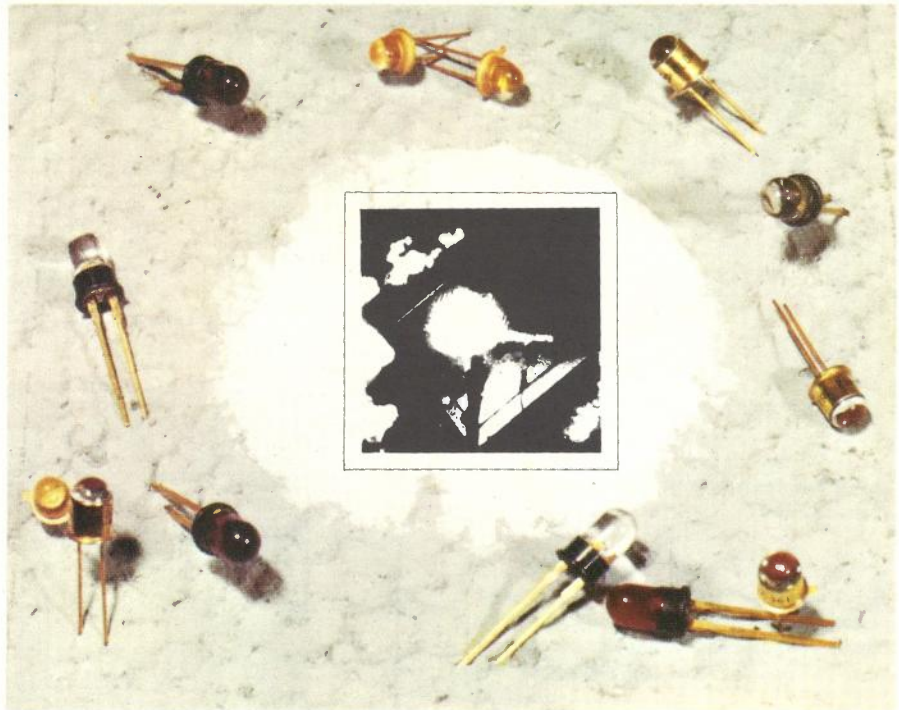
AN ARRAY OF L.E.D. INDICATORS CENTRE INSET: L.E.D. CHIP PHOTOGRAPHED USING ITS OWN LIGHT
