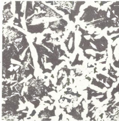
MICROSTRUCTURE OF STEEL FROM MAST THAT FAILED
