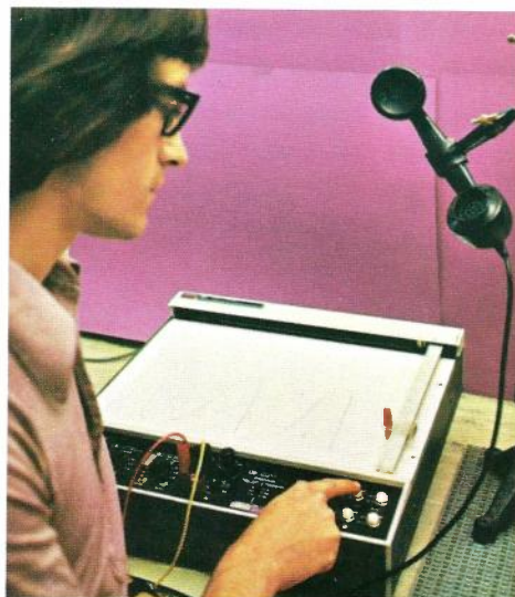
A CARBON MICROPHONE IS TESTED FOR D.C. CURRENT STABILITY
