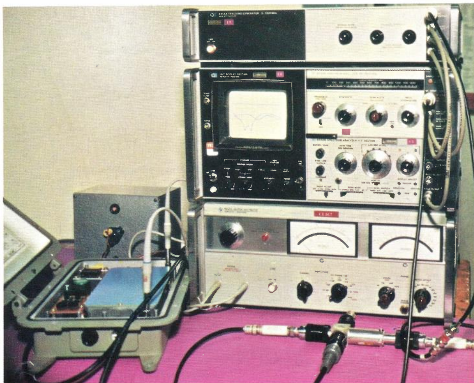
COMMERCIAL CTV MAIN ROUTE AMPLIFIER UNDERGOING SWEPT FREQUENCY RETURN LOSS MEASUREMENTS
