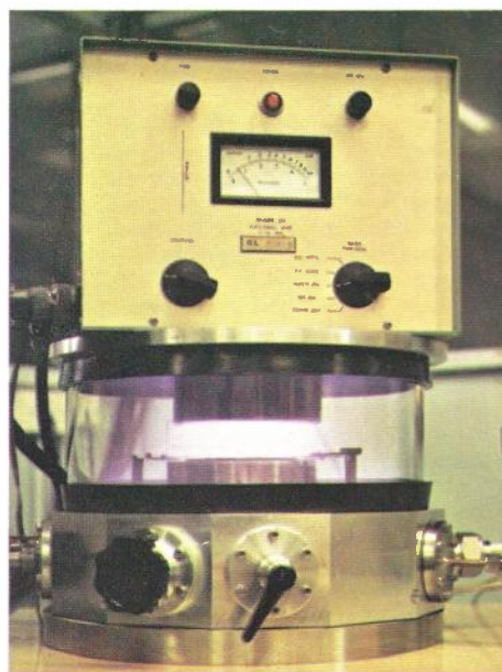
RF PLASMA SPUTTERING FACILITIES FOR LED SOURCES.
