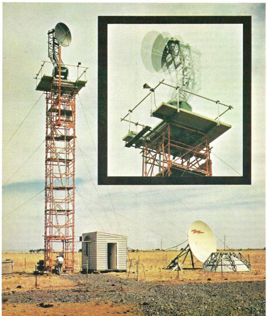
THE RECEIVING END AT THE OUTDOOR ANTENNA TEST RANGE INSERT: ANTENNA UNDER TEST MOUNTED ON THE REMOTELY CONTROLLED ELEVATION-ON-AZIMUTH ANTENNA POSITIONER
