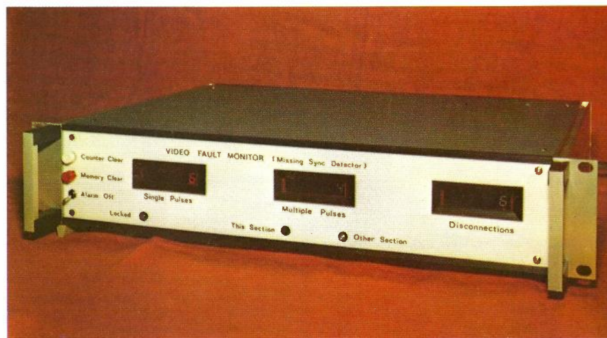
▼ Experimental instrument for classifying and counting interruptions in video signals
