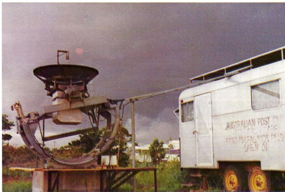
The Darwin 11 and 14 GHz radiometer - about to measure some heavy rain attenuation
