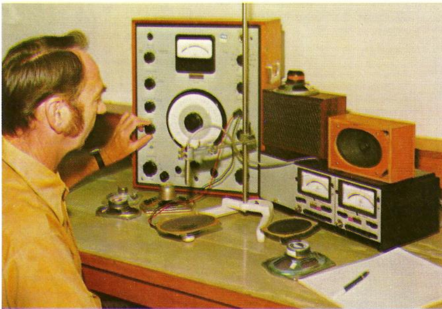
"Close field" testing of loudspeakers permits their evaluation on a laboratory bench
