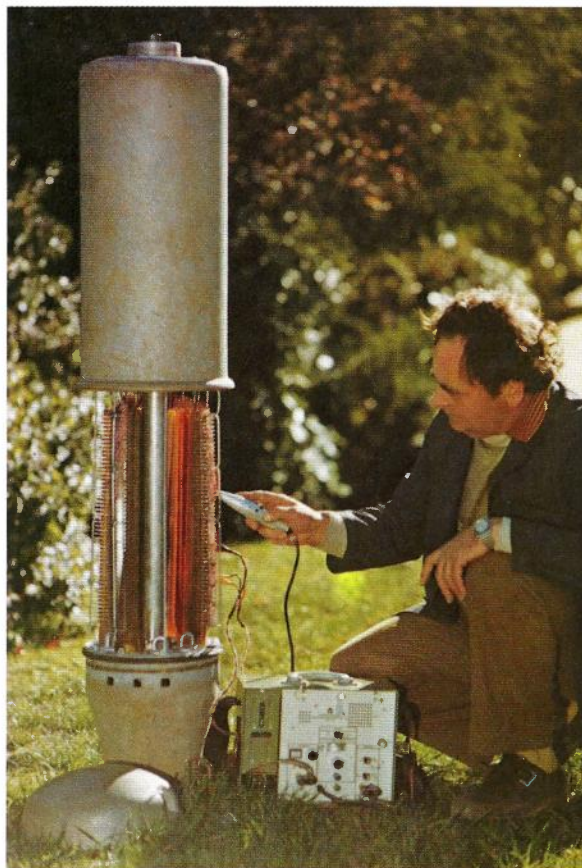
The general purpose cable identification set with search probe being moved over the pairs to identify them
