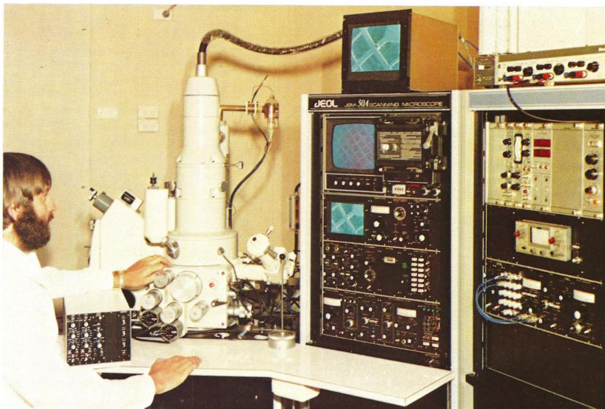
Scanning electron microscope showing a secondary electron image of an etched microgrid
