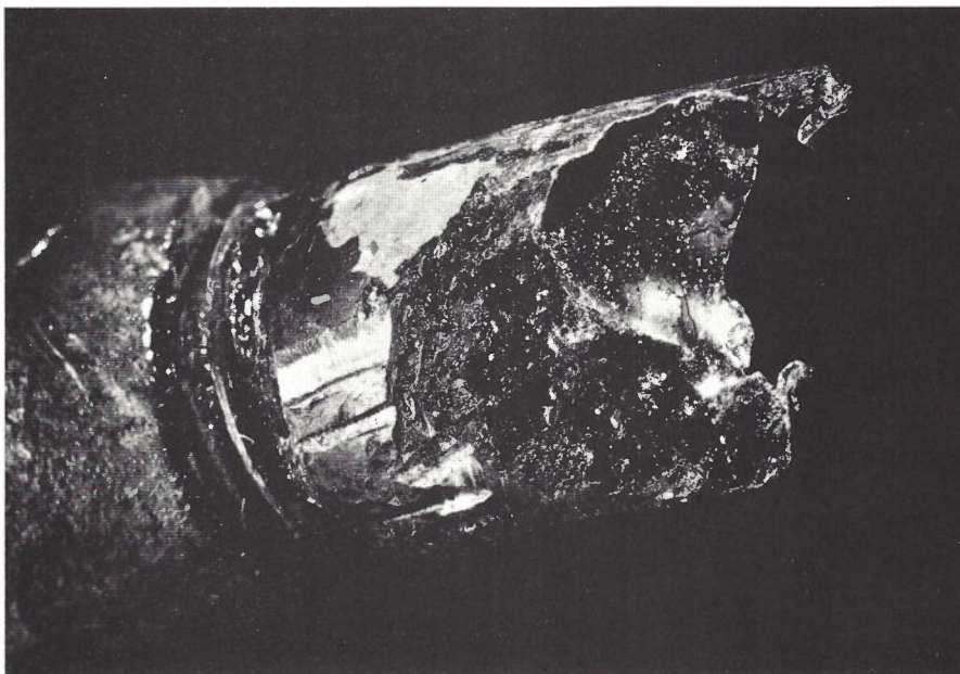
A copper bit after 600 operations using a tin/lead solder (60/40)
