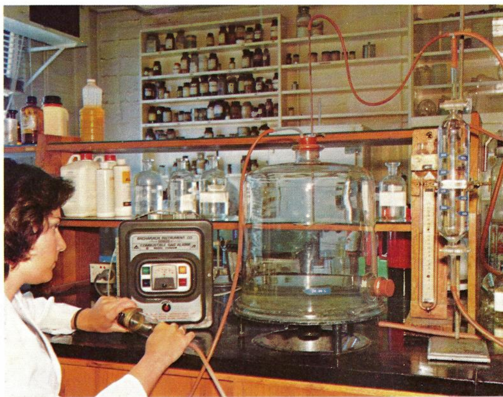
Apparatus to determine the response characteristics of combustible gas detectors
