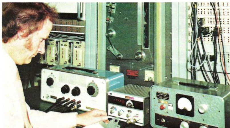
Measuring echo path loss using pink noise
