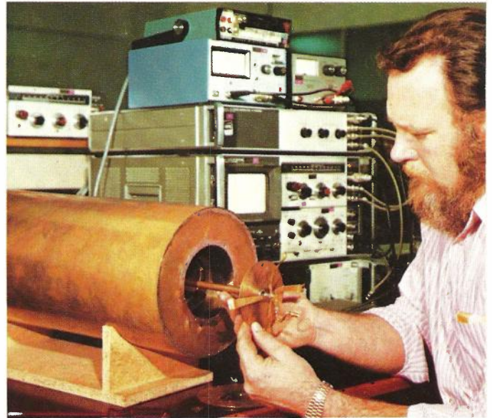
Ready interchangeability of cable test samples is a feature of the Quintaxial test fixture
