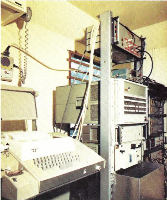
Left: Receiving equipment van showing minicomputer and peripherals
