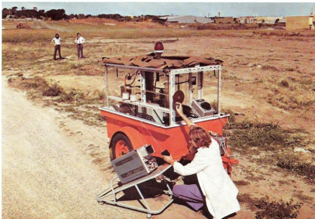
The impulse generator being used to measure earth parameters using a high voltage pulse
