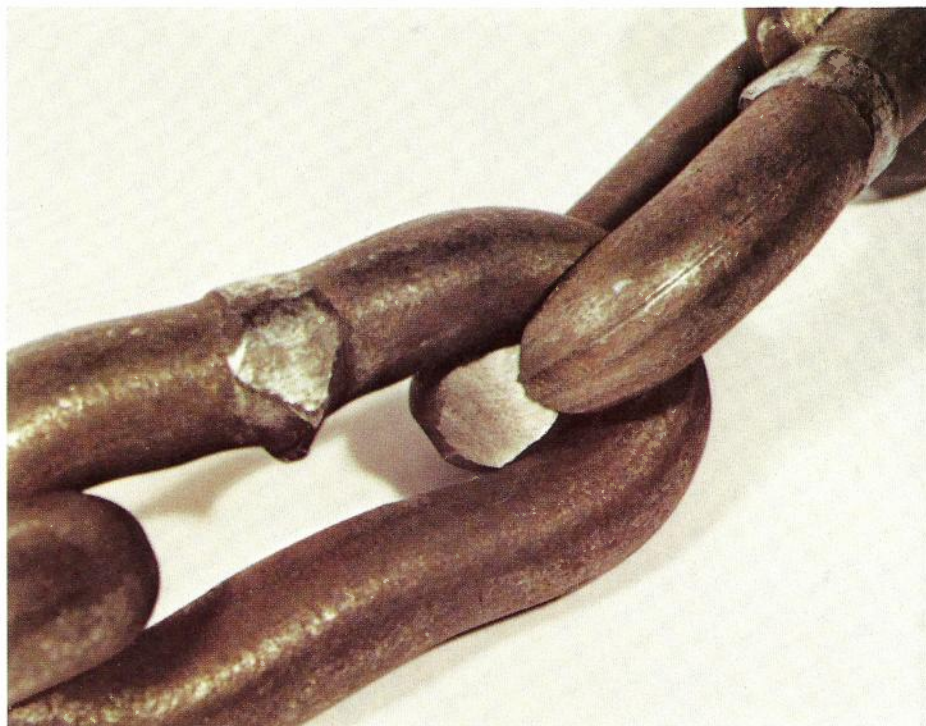
Failed link in chain
