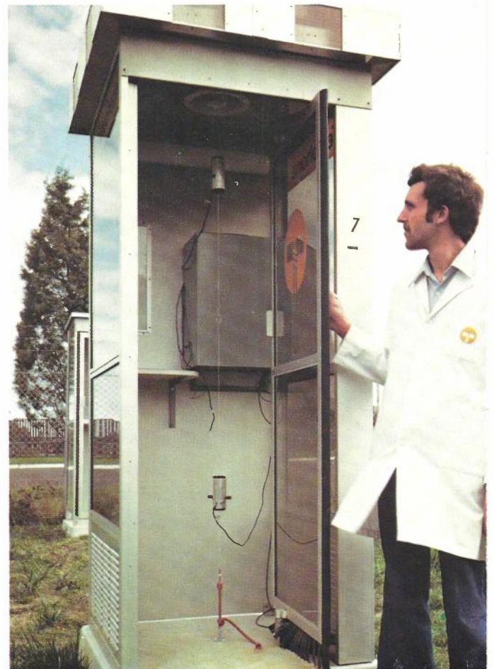
CW520 cabinet fitted with louvers, insulation, tinted glass and fan
