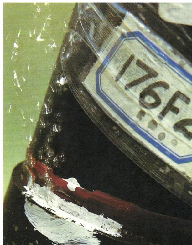
Heat-shrinkable Cable End Seal immersed in water showing air escaping from faulty joint
