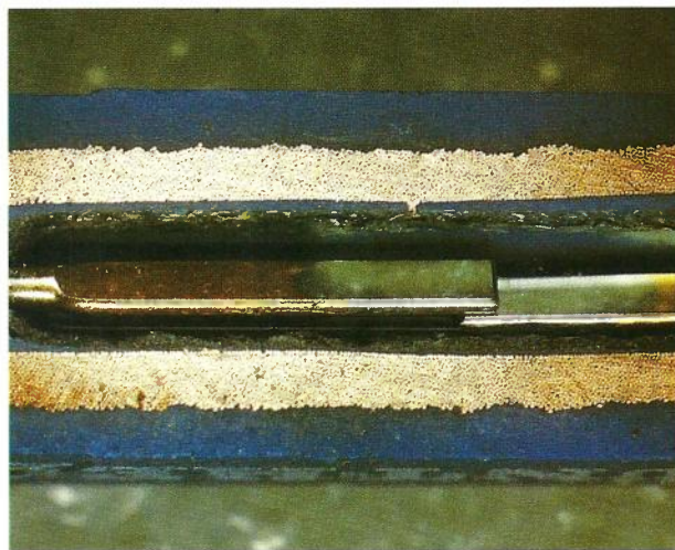
Magnified view of contact set of miniature relay
