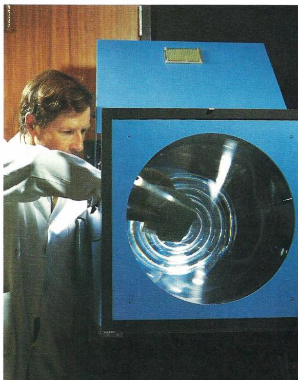
Light source of pulsed solar simulator showing coiled Xenon arc tube through the Fresnel lens
