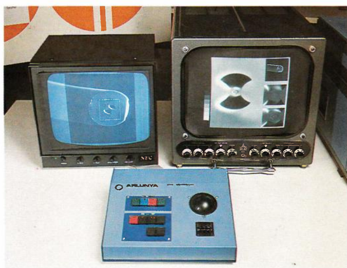
Right hand screen of image processing system shows composite picture of polarisation-preserving fibre after various stages of etching
