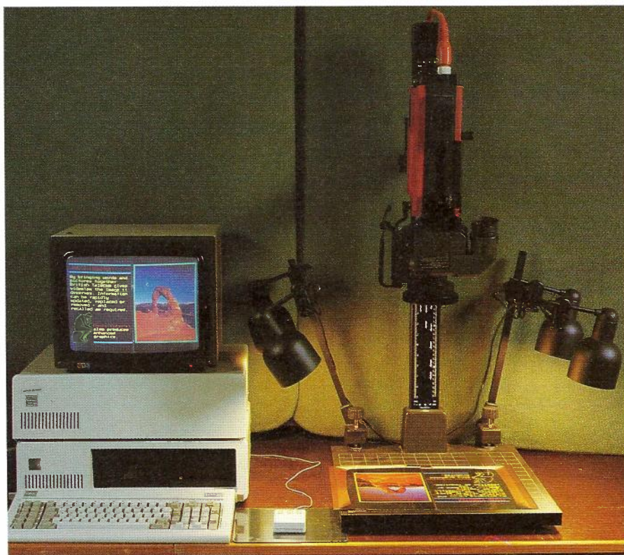
Demonstration photo videotex system using the 64 kbit/s connection capability of the ISDN testbed
