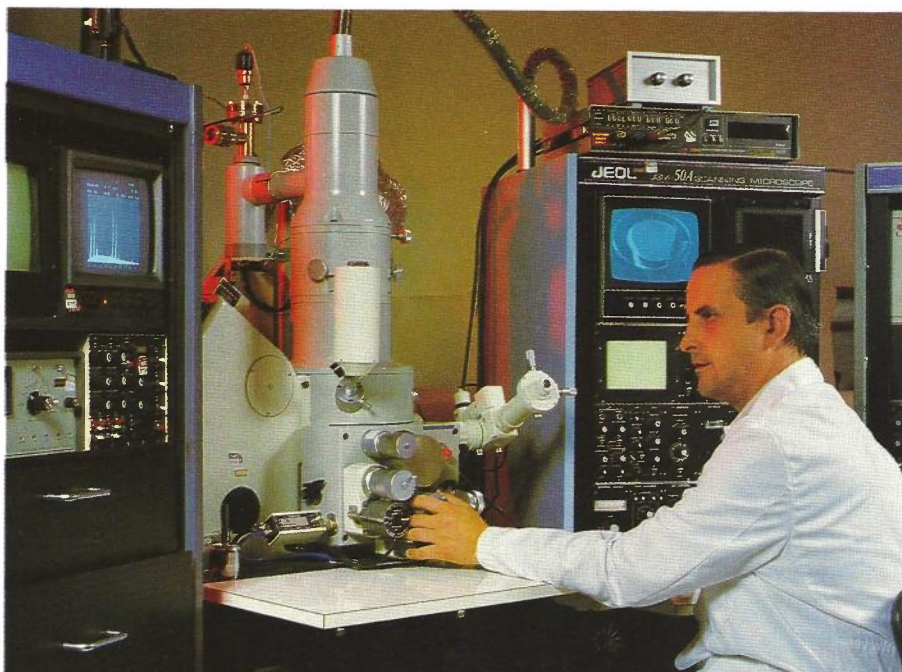
Electron probe micro-analysis system applied in characterising new glasses for optical fibres
