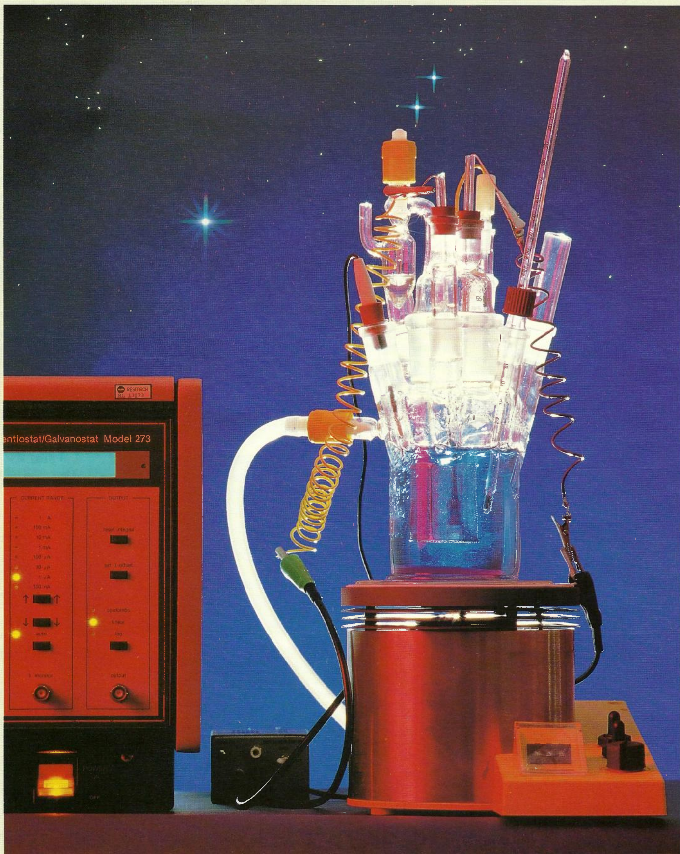
Multi-ported electro-chemical cell for characterising tellurium and cadmium compounds
