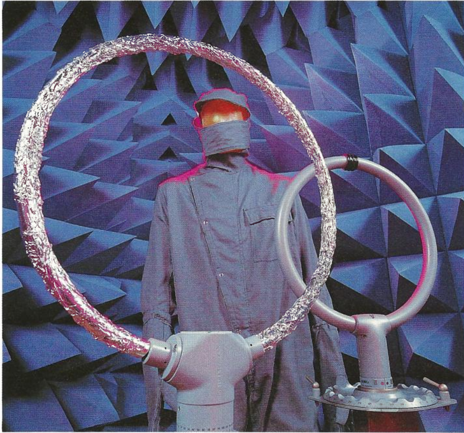
The RF protective suit, showing its open face
