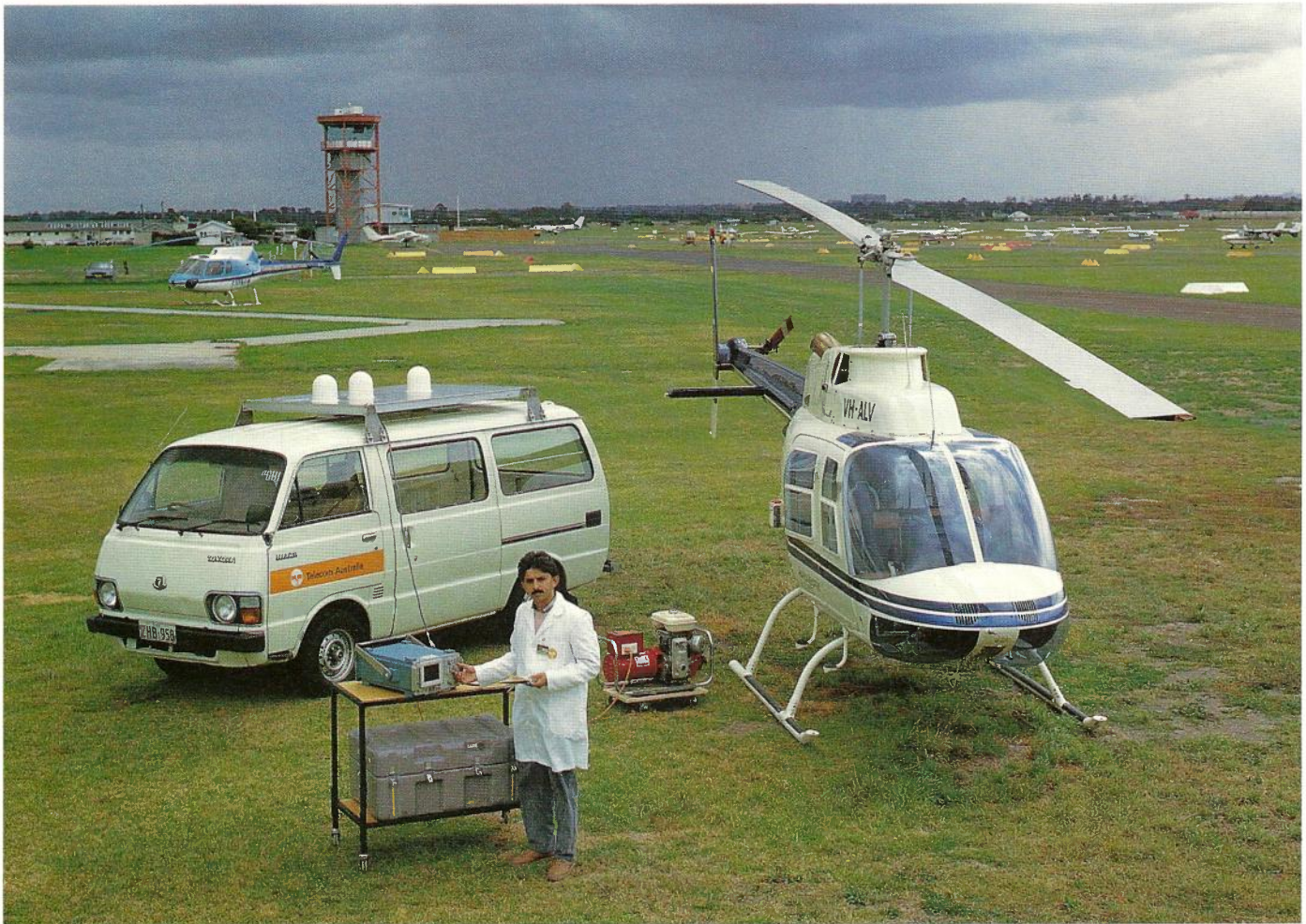
The instrumented helicopter and vehicle used to simulate earth-space propagation effects in satellite-based mobile services
