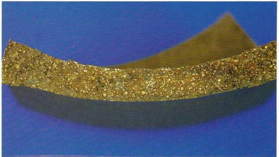
Stress corrosion cracking in a waveguide connector casting
