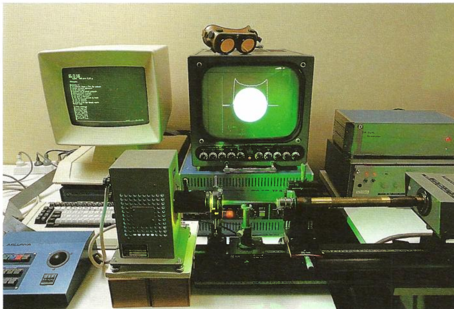
The Laboratories' experimental facility for characterising optical fibres by refractive index profile using near-field intensity scanning techniques
