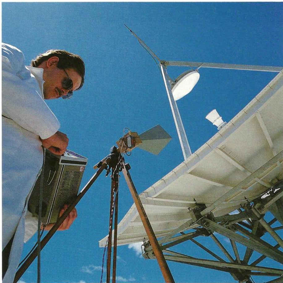
The tripod-mounted portable test cell used in electromagnetic field measurements
