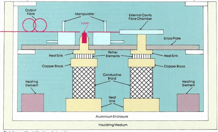
Block diagram of the stabilised laser diode module.
