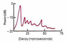
Typical delay spread profile of a radio path in a wire-less office environment.
