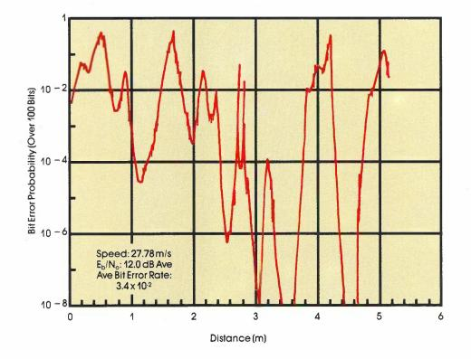
Variation of bit error probability over a 5 m distance travelled by a mobile receiver in a typical urban mid-block location. transceiver moves through its environment. The performance of six modulation schemes are being studied, namely, the coherent and differential forms of each of:
