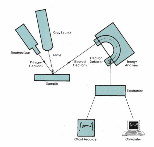
Schematic representation of the components necessary for X-ray Photoelectron Spectroscopy and Scanning Auger Microanalysis.
