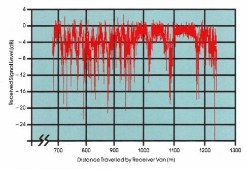
Simulated mobile earth-to-space propagation results
