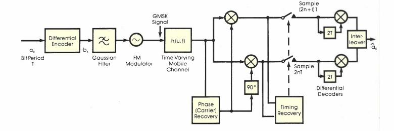
Schematic outline of a transmission system employing Gaussian Minimum Shift Keying (GMSK) modulation.
