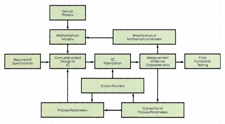
An illustration of the iterative process involved in the fabrication of integrated circuit devices.
