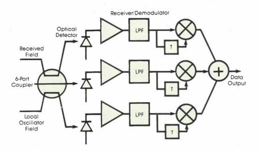
Schematic diagram of the optical phase-diversity receiver.
