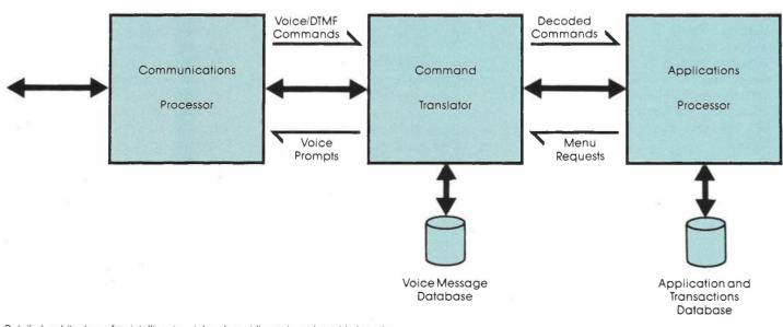
Detailed architecture of an intelligent peripheral providing voice value added services.
