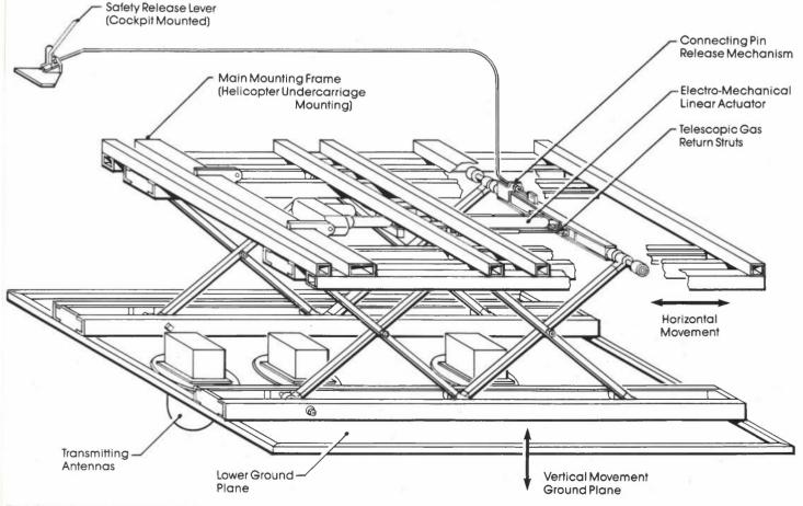
The Laboratories-designed helicopter antenna mount.
