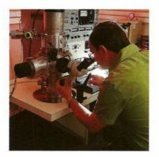
equipment is also equipped with a cooled specimen stage to prevent the specimens heating during the thinning process, since high temperatures may result in modification of the interfaces being investigated.
