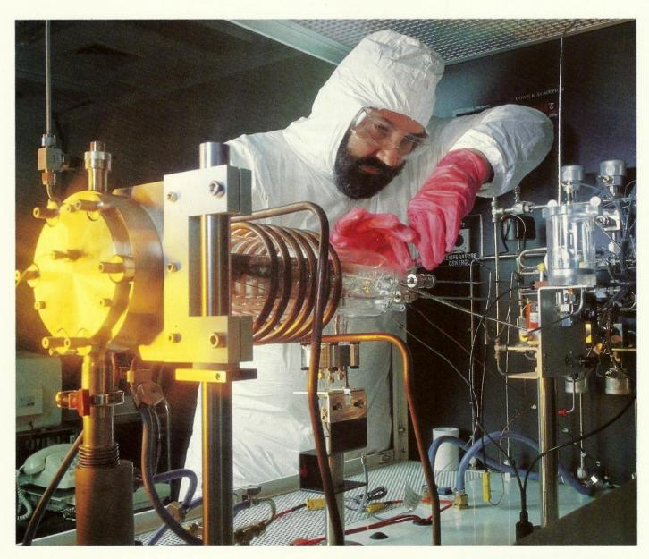
The reactor itself contains a resistively heated mercury pool and an RF inductively heated susceptor on which the substrates are placed. The various deposition parameters such as gas flow rates, flow times and reactor temperatures are precisely controlled and monitored by a microprocessor-based control system. This system also ensures that the system automatically shuts down in a safe mode should any fault occur during the process.
