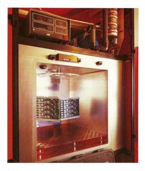
The role of water vapour in the surface corrosion process is considered to be crucial and proposed new standard test atmospheres demand high relative humidity, controlled to tighter limits.
