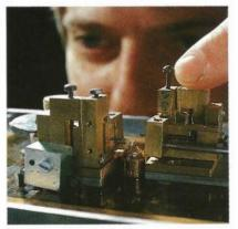
Linewidth reduction has been achieved in the laboratory by the use of an external cavity to introduce weak optical feedback to the laser diode. These external cavities consist of a short length of temperature controlled optical fibre with a mirrored endface. With this configuration, about a one thousand fold reduction of spectral linewidth has been achieved. Measurement of the narrow linewidth is performed using the delayed selfheterodyne technique.
