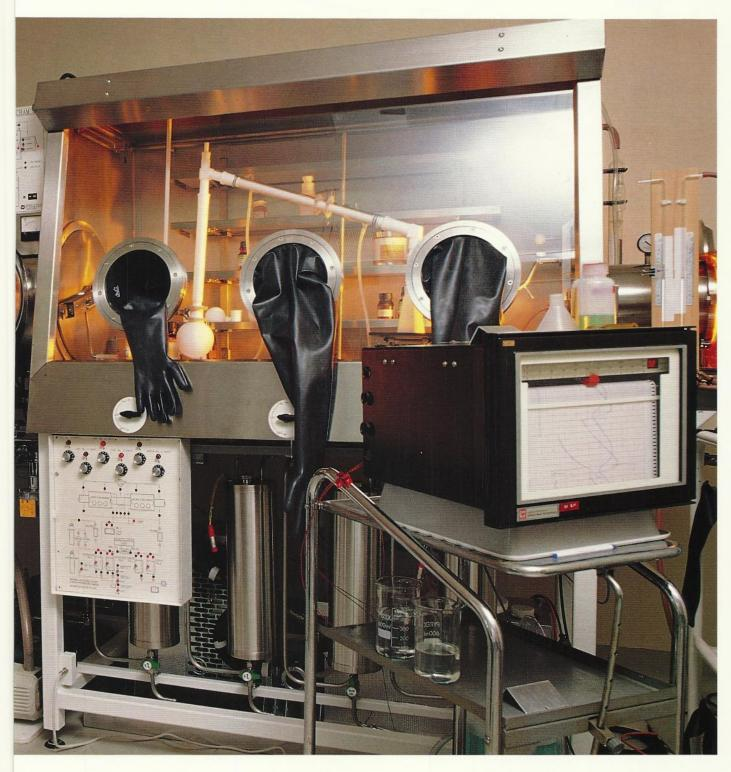
**Above** The award-winning Recirculating Inert Atmosphere Chamber designed and built in the Laboratories
