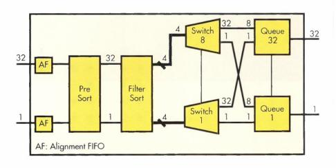
**Above** A 32 x 32 self-routing switch fabric with 8 parallel stages
