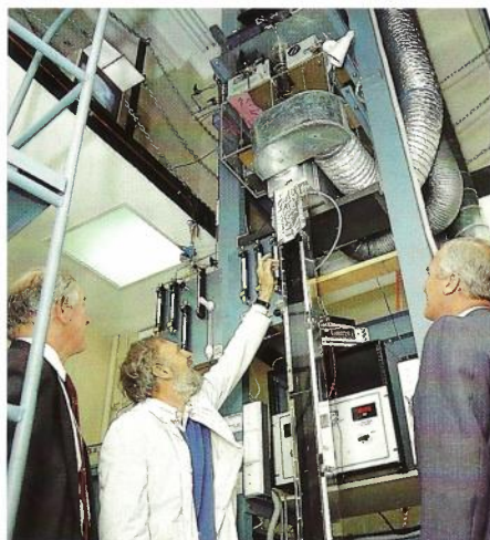
Researcher Dr Gavern Rossman demonstrates TRL's optical fibre drawing tower to Frank Blount and Harry Wragge.
