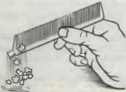
FIG. 7. ELECTRIC FORCE OF ATTRACTION.
