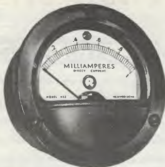
(a) Typical Moving Coil Instrument.
