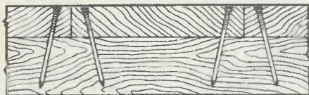
METHOD OF NAILING TO OBTAIN BETTER GRIP
