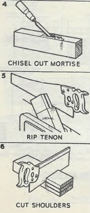
FIG. 1. CONSTRUCTION AND APPLICATION OF MORTISE AND TENON JOINTS.
