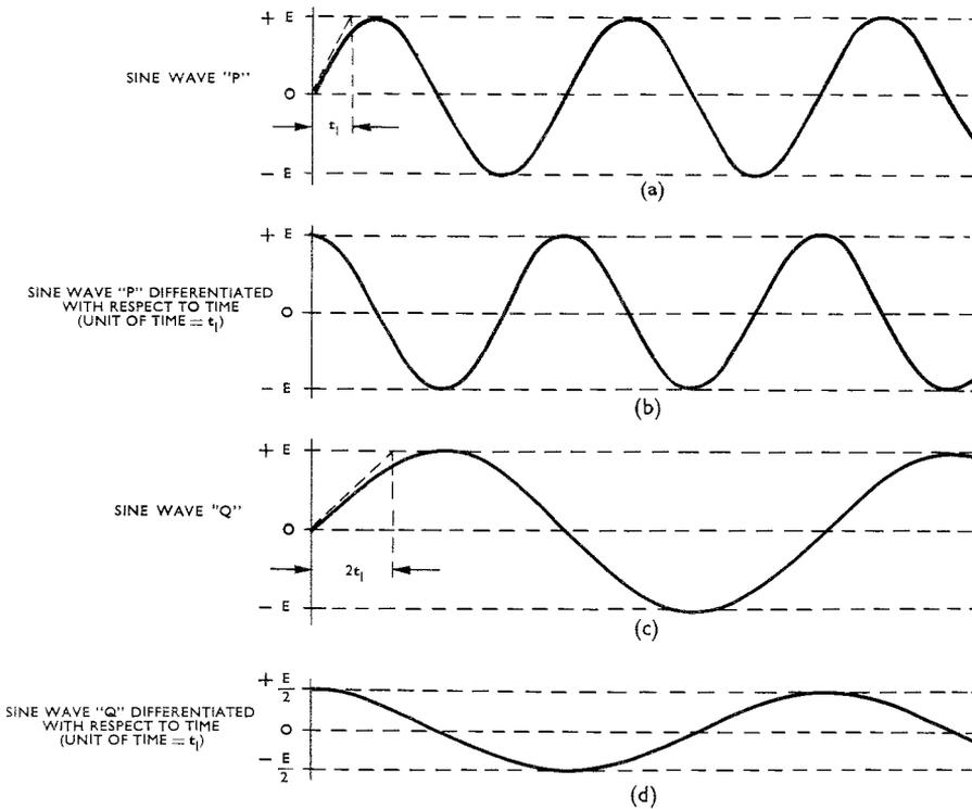
FIG. 26. AMPLITUDE OF DIFFERENTIATED SINE WAVE.
