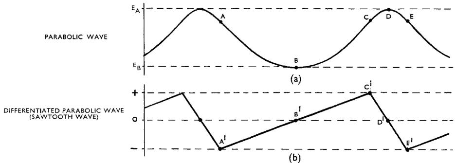
FIG. 24. DIFFERENTIATION OF A PARABOLIC WAVE.
