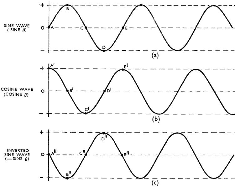
FIG. 25. DIFFERENTIATION OF A SINE WAVE.
