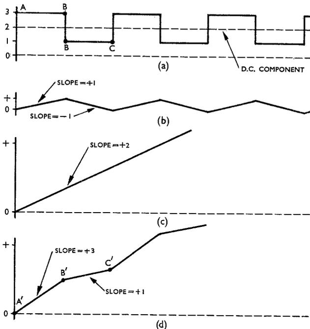
FIG. 37. INTEGRATION OF A D.C. COMPONENT.
