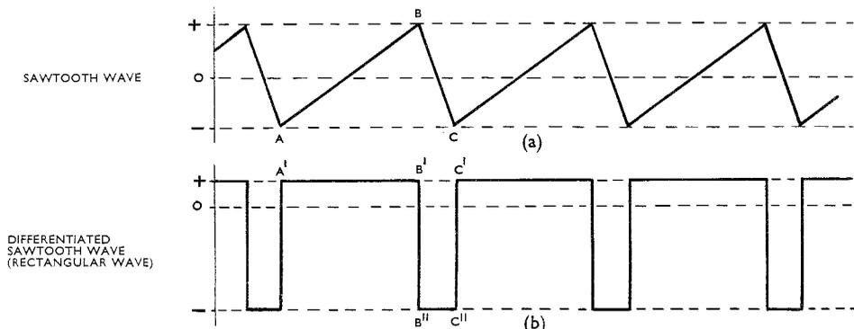
FIG. 23. DIFFERENTIATION OF A SAWTOOTH WAVE.
