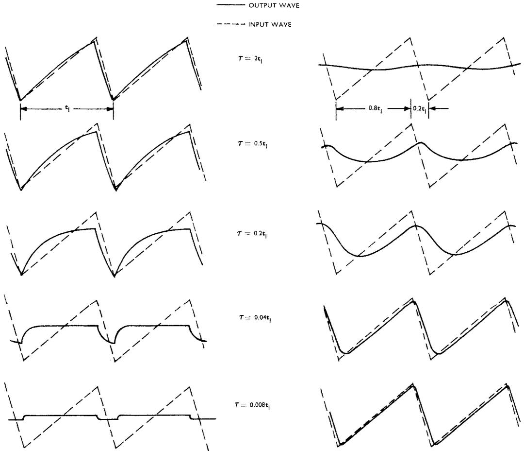
(a) Resistor Voltage Waveforms ( $e_R$ ).
