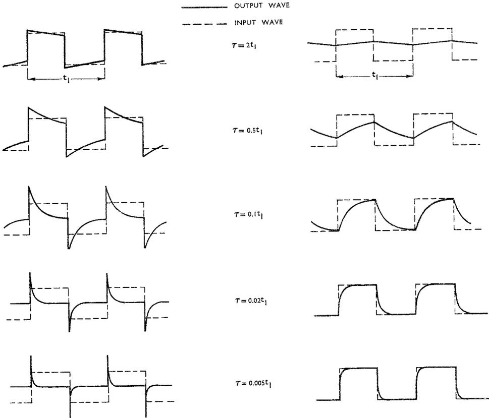
(a) Resistor Voltage Waveforms ( $e_R$ ).
