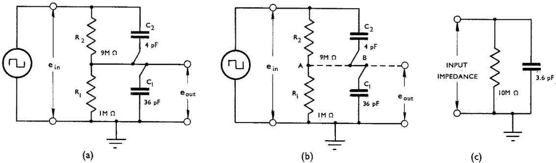
FIG. 44. COMPENSATED VOLTAGE DIVIDER.
