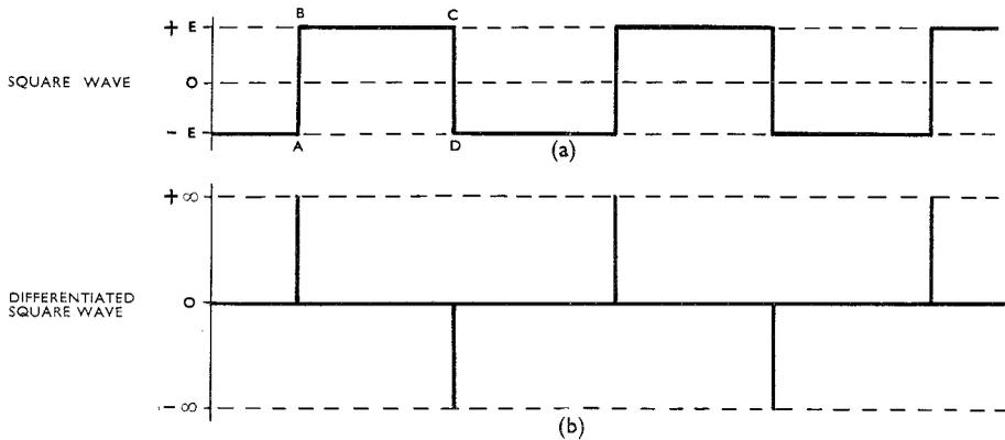
FIG. 22. DIFFERENTIATION OF A SQUARE WAVE.
