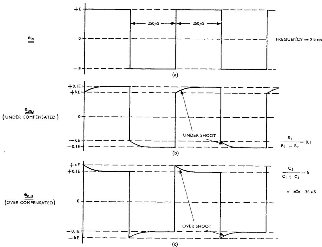
FIG. 45. INCORRECTLY COMPENSATED VOLTAGE DIVIDER.
