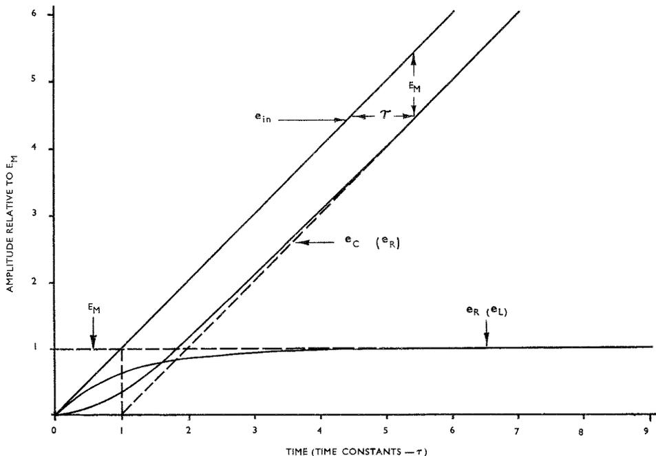
FIG. 6. CONSTANTLY INCREASING VOLTAGE INPUT TO R-C CIRCUITS.
