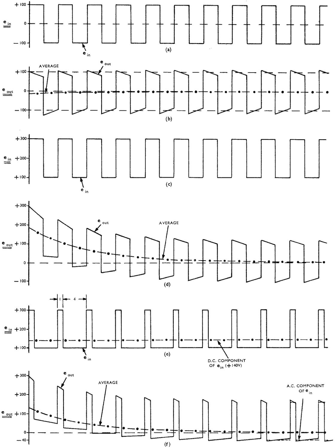
FIG. 14. COUPLING CIRCUIT OUTPUT WAVEFORMS.
