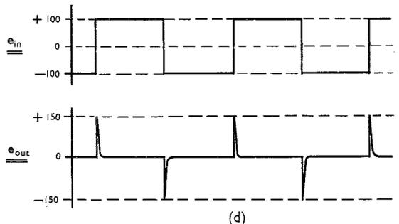
FIG. 33. EFFECT OF CAPACITIVE LOAD ON A DIFFERENTIATING CIRCUIT.
