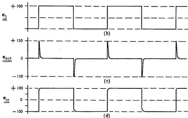
FIG. 32. EFFECT OF SOURCE RESISTANCE.
