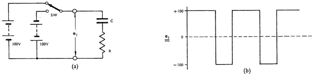
FIG. 1. CIRCUIT PRODUCING RECTANGULAR WAVE INPUT.
