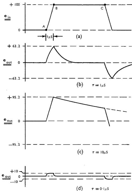
FIG. 31. DIFFERENTIATION OF "RECTANGULAR" WAVES WITH A FINITE RISE TIME.
