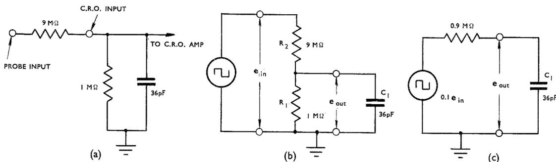
FIG. 43. UNCOMPENSATED VOLTAGE DIVIDER.
