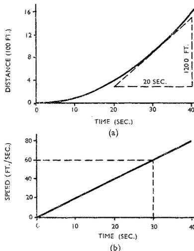
FIG. 18. DIFFERENTIATION OF A PARABOLIC CURVE.
