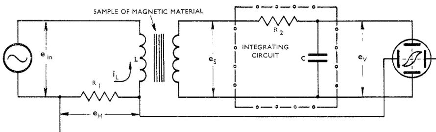
FIG. 42. MAGNETIZATION CURVE DISPLAY USING INTEGRATING CIRCUIT.
