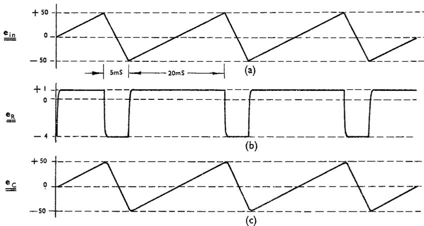
FIG. 8. SAWTOOTH WAVES IN SHORT TIME CONSTANT R-C CIRCUIT.
