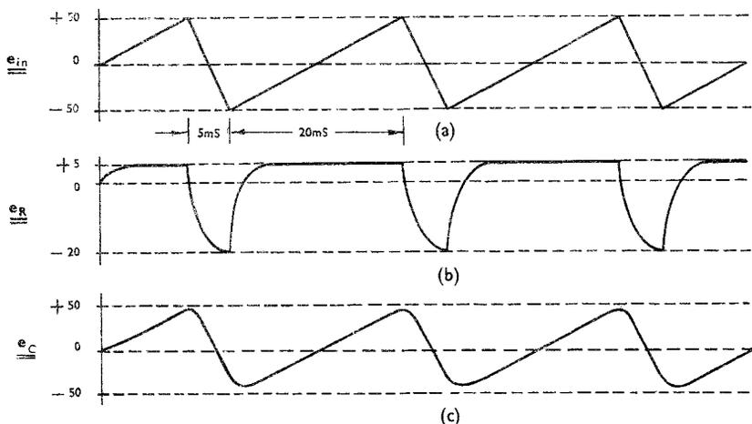
FIG. 7. SAWTOOTH WAVES IN MEDIUM TIME CONSTANT R-C CIRCUIT.
