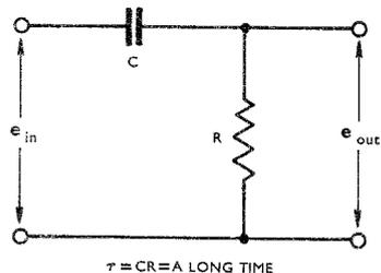
FIG. 12. COUPLING CIRCUIT.
