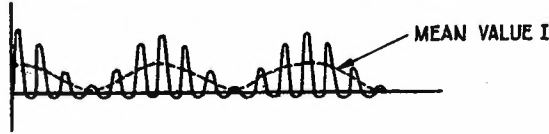
(b) Distorted Radio-Frequency Output from a Detector Stage of a Receiver (Showing Fluctuating Mean).
