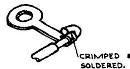
FIG. 16. POWER TYPE TERMINAL.
