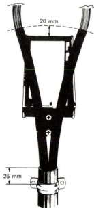
Attaching Cover Chain MOUNTING BOX ON POLE
