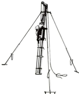
ROD DRIVING JIG (S446/8) FITTED WITH "COBRA" HAMMER
