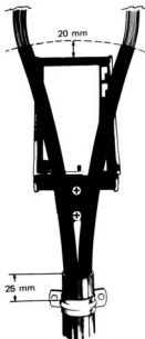
Marking Coach-screw Positions
