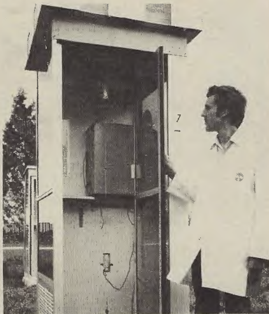
Experimental phone cabinet fitted with louvres, insulation, tinted glass, fan and monitoring instruments.
