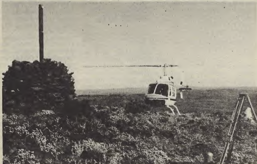
Helicopter ferries surveyors and their equipment between the site on the summit of Mt Dering and the road below. Picture shows a trig station (left) and a surveyor's tripod.
