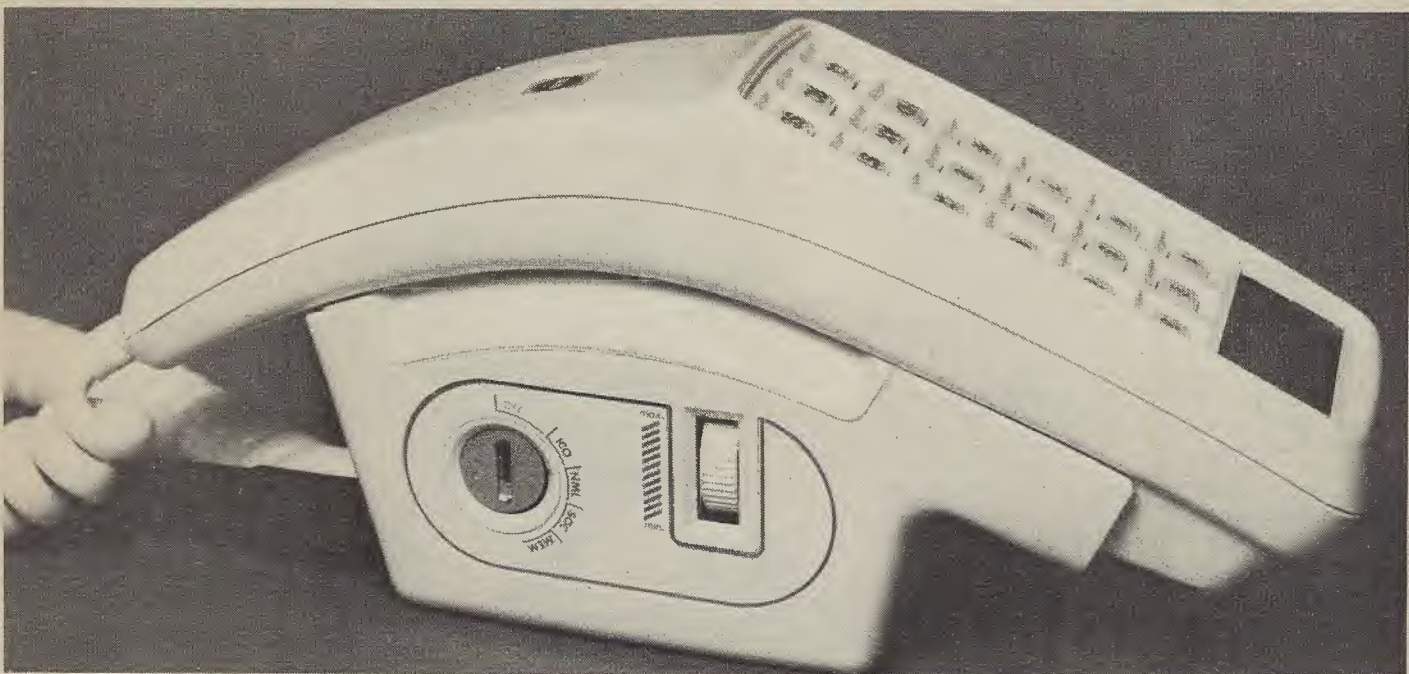
Handpiece and cradle of Australia's first automatic mobile telephone set showing function and dial buttons and dialled numbers display. On the cradle is seen locking and control key and speaker volume control.
