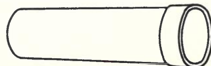
Fig. 2.—Lead Sleeve with Brass Reinforcing Collar.
