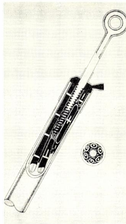
Fig. 5.—Epoxide Resin Pulling Termination for Coaxial Cable.
