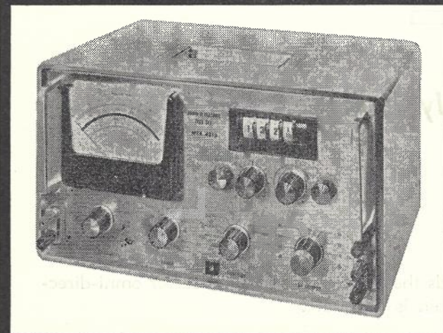
M.T.S. A210—Audio/Ultrasonic Test Set for the complete evaluation of audio and ultrasonic amplifiers, filters and transmission circuits.
