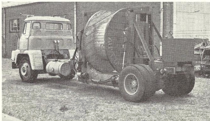
Fig. 2.—7 Ton Capacity Cable Drum Transporter.
