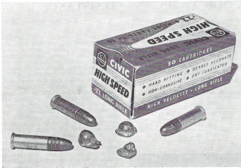
Fig. 2 — Cartridges used in Tests and Examples of Deformer Bullets after Testing.
