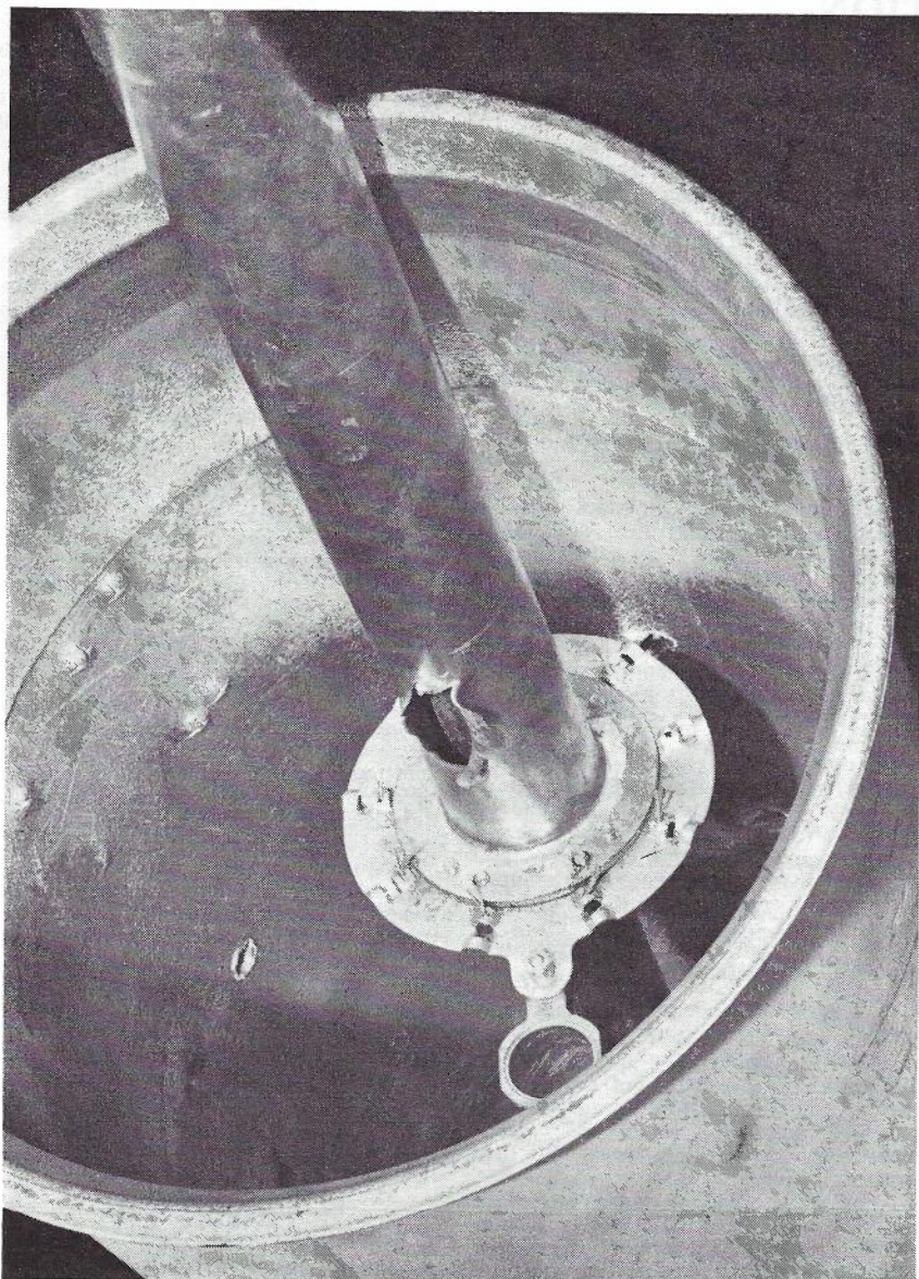
Fig. 6 — Inside Surface of a 900 Pair Cover, showing Star Shaped Cracks from Bullet Penetration.
