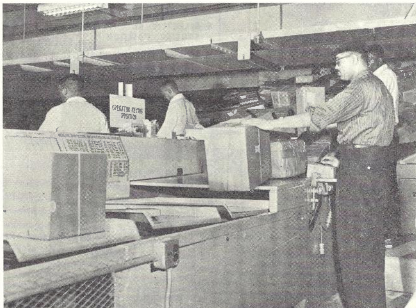
Fig. 9 — Parcel Sorting Machine — Using Tilted Tray Method for Parcel Diversion — U.S. Post Office.
