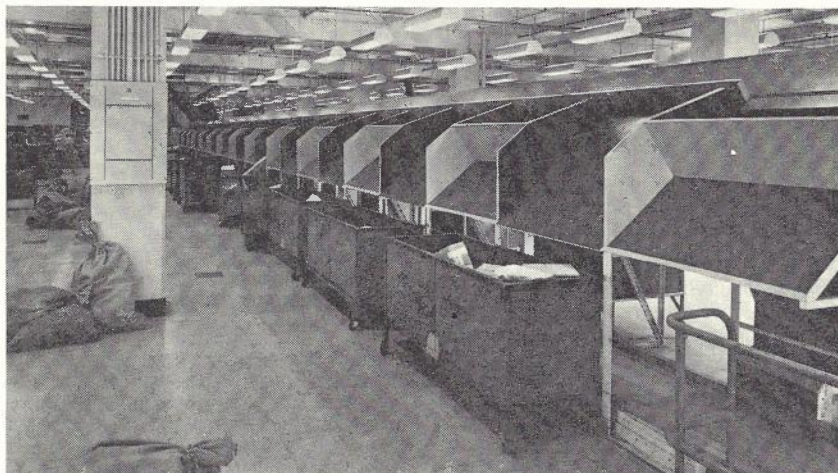
Fig. 7. — Country Parcel Secondary Sorting Machine Sloping Belt Section.
