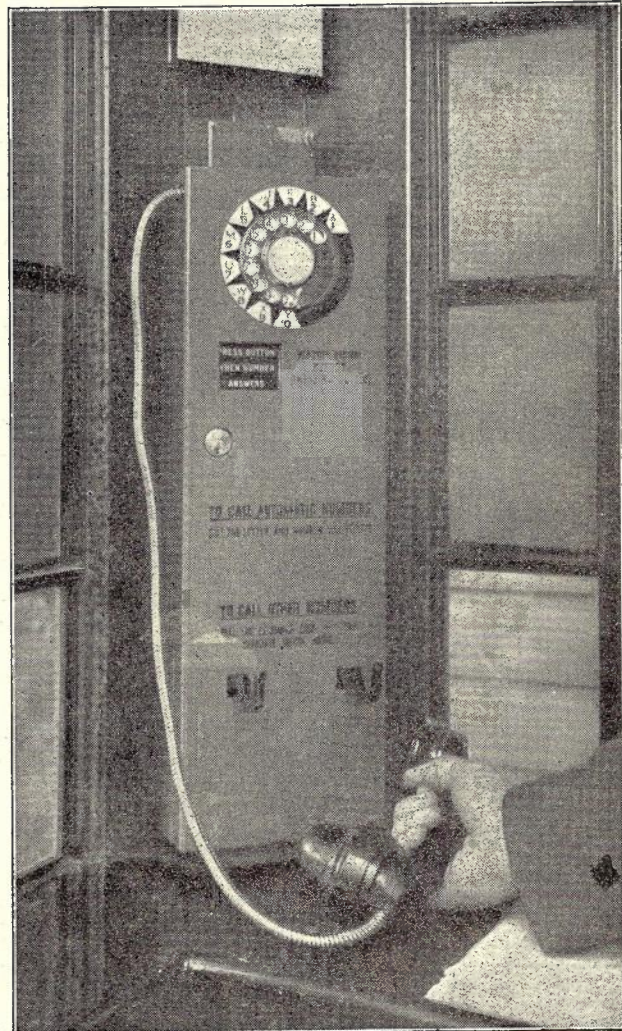
Fig. 6.—Corner Type Public Telephone.
