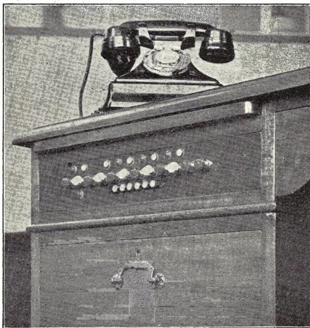
Fig. 2.—Drawer Unit with Vertical Key Panel.
