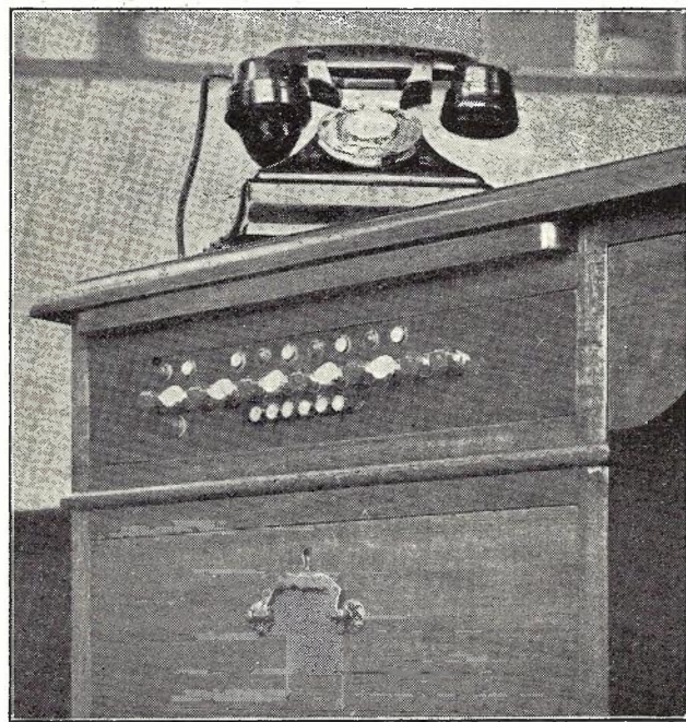
Fig. 2.—Drawer Unit with Vertical Key Panel.
