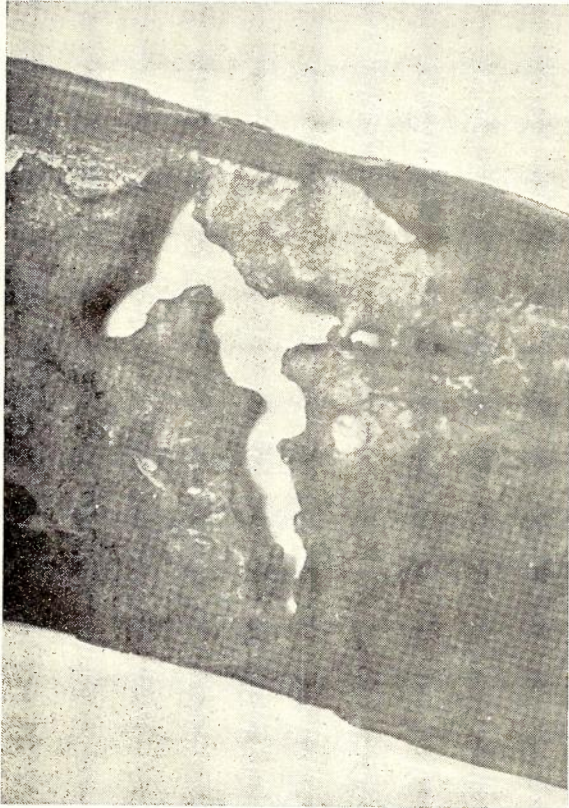
Fig. 2.—Photograph of Damaged Cable Sheathing showing Hole made by Singapore Ants. Magnification 4.5.
