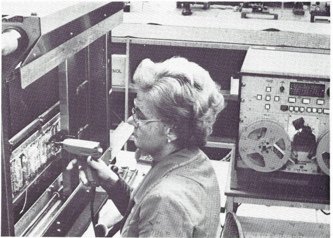
Assembly of the Mothercard by the Australian Electronics Industry for the Minicomputer of the Australian Designed and Manufactured Traffic
