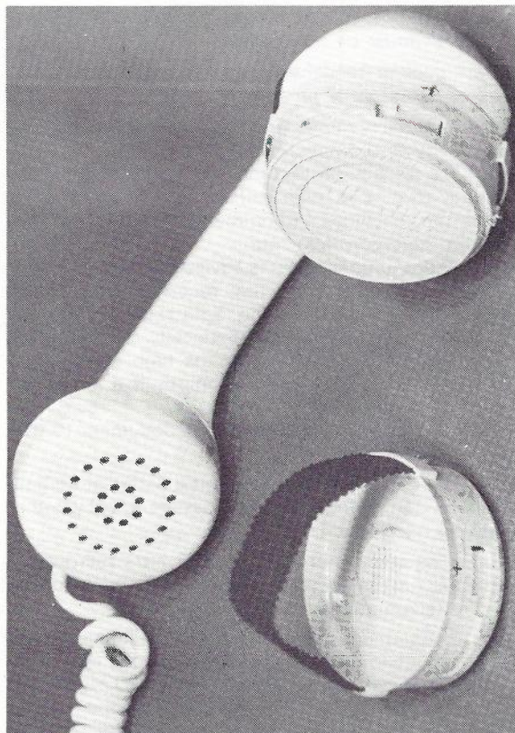
The new hearing aid coupler detached (lower) and fitted to a telephone handset. The coupler is intended to be used with modern ear-level hearing aids.
