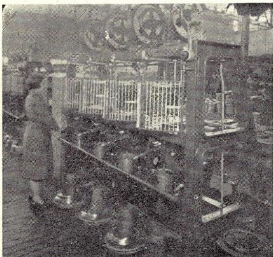
Fig. 6.—Four-head trunk cable insulating machine.
