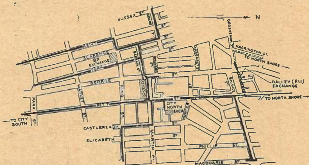
Fig. 1.—New Dalley Tunnel (shown thick dotted line) in relation to existing tunnel (shown thick full line).
